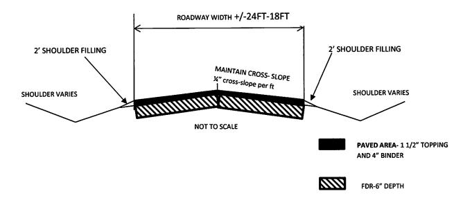
FDR WILL BE +/-24FT-18FT AND 6" DEPTH. MAINTAIN PROPER CROSS SLOPE FOR DRAINAGE. RESURFACE FULL WIDTH WITH 440LBS PER SQUARE YARD RECYCLED ASPHALTIC CONCRETE 19MM SUPERPAVE, GP 2 ONLY, INCL BITUM MATL & H LIME AND 165LBS PER SQUARE YARD RECYCLED ASPHALTIC CONCRETE 12.5MM SUPERPAVE, GP 2 ONLY, INCL BITUM MATL & H LIME
