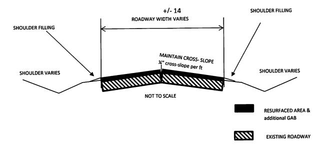
MAINTAIN PROPER CROSS SLOPE. GRADE AND PREP BASE WITH ADDITIONAL 220 LBS OF GAB W/PRIME OR AS DIRECTED BY ENGINEER. RESURFACE APPROXIMATELY +/-14 FT WIDTH WITH 220 LBS PER SQUARE YARD RECYCLED ASPHALTIC CONCRETE, 12.5MM SUPERPAVE, GP 2 ONLY, INCL BITUM MATL & H LIME.
